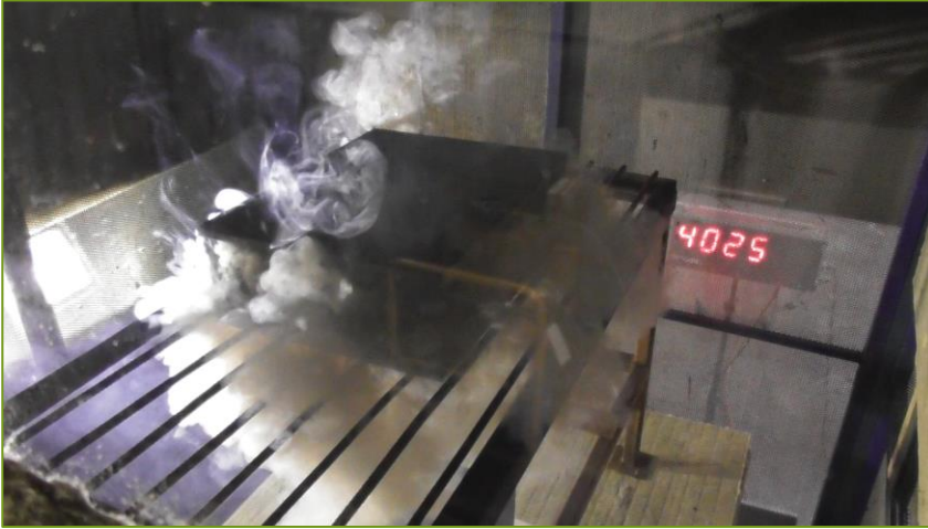
Thermal Runaway off-gas from a battery module
