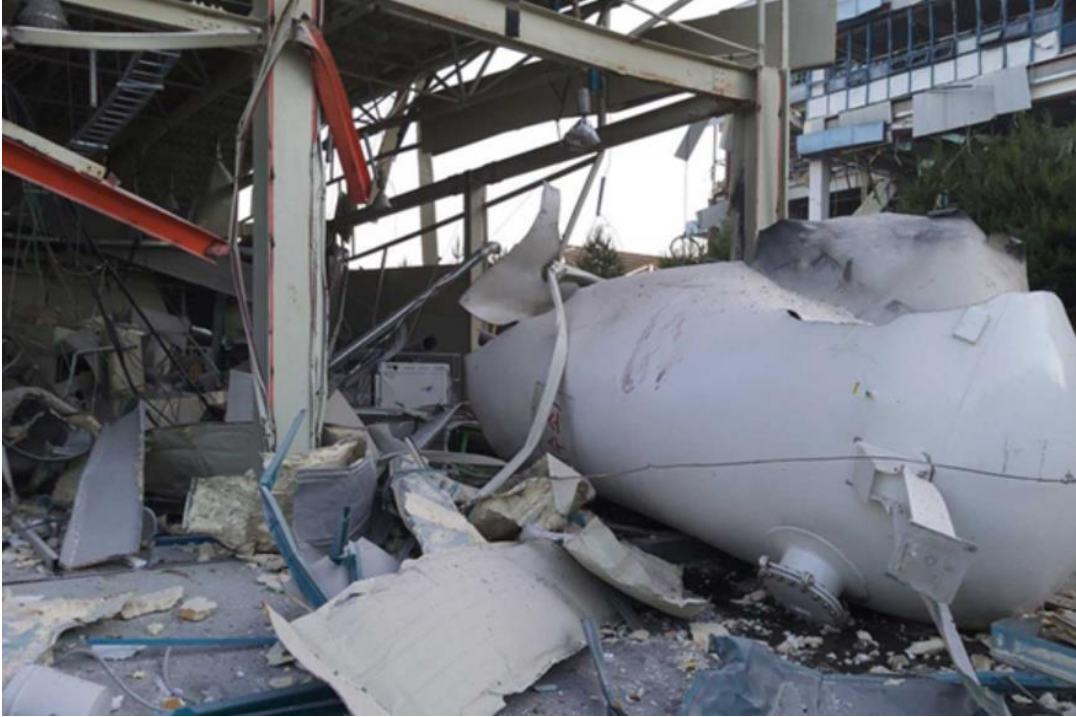
In Equipment Explosion : AEME research facility South Korea 2 men died and several buildings 100 meters away have been seriously damaged
