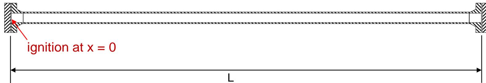
**1<sup>st</sup> step:** trigger an explosion with transition to detonation inside a pipe
