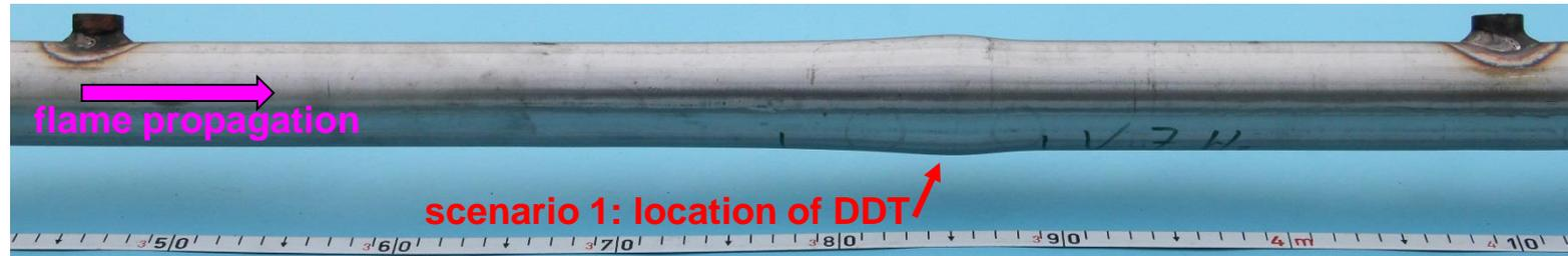
**Test 19:** 10 bar abs, 20 °C, CH<sub>4</sub> : O<sub>2</sub> = 11.25 : 88.75 [vol.-%], 48.3 x 2.6 pipe, material: 1.4541
