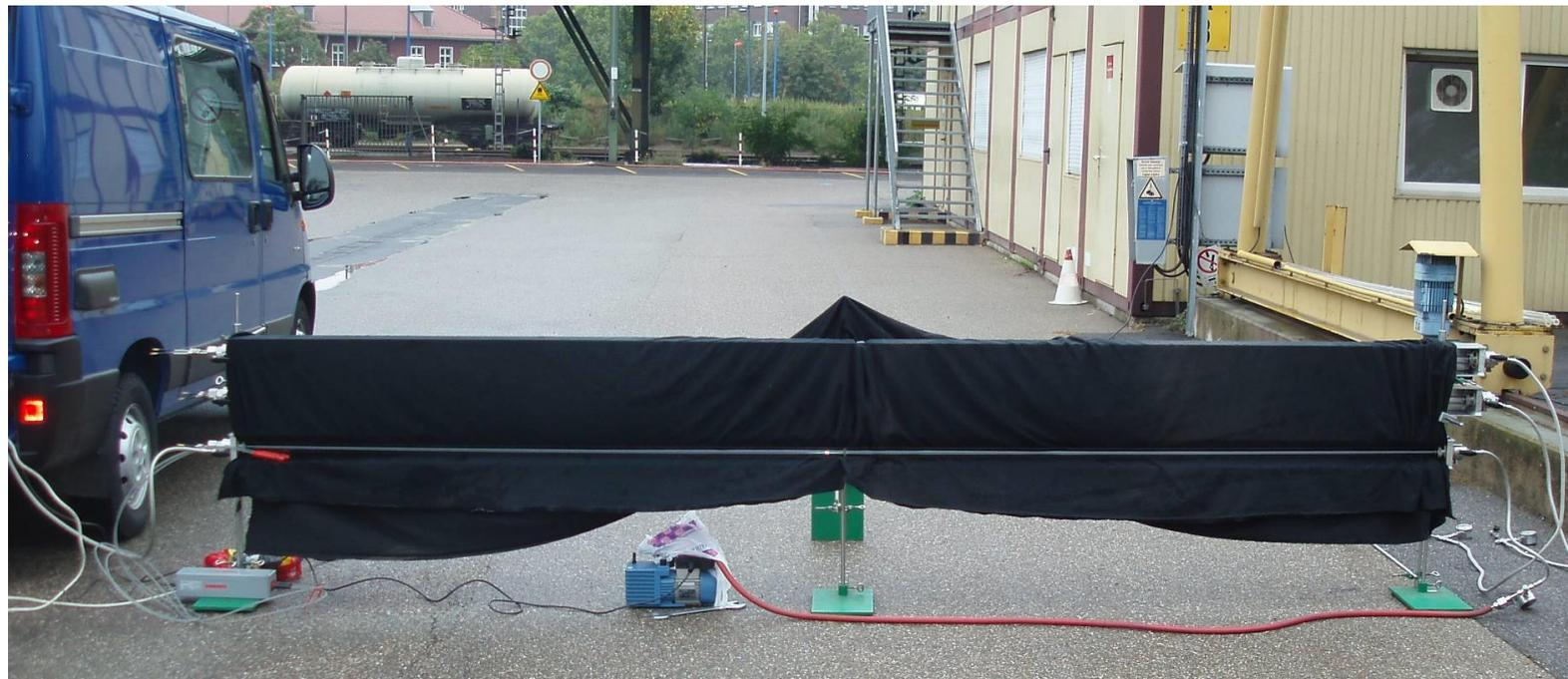
Deflagration to Detonation transition in almost stoichiometric propane/air-mixture at about  $90 \cdot \phi_i$  distance to point of ignition (=1.8 m), 3 bar abs, 15°C, pipelength = 4 m,  $\phi_i = 20$  mm
