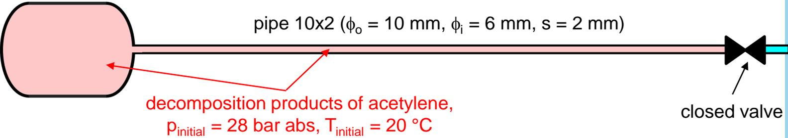
**Case 1:** pipe length is 1.5 m: no rupture
