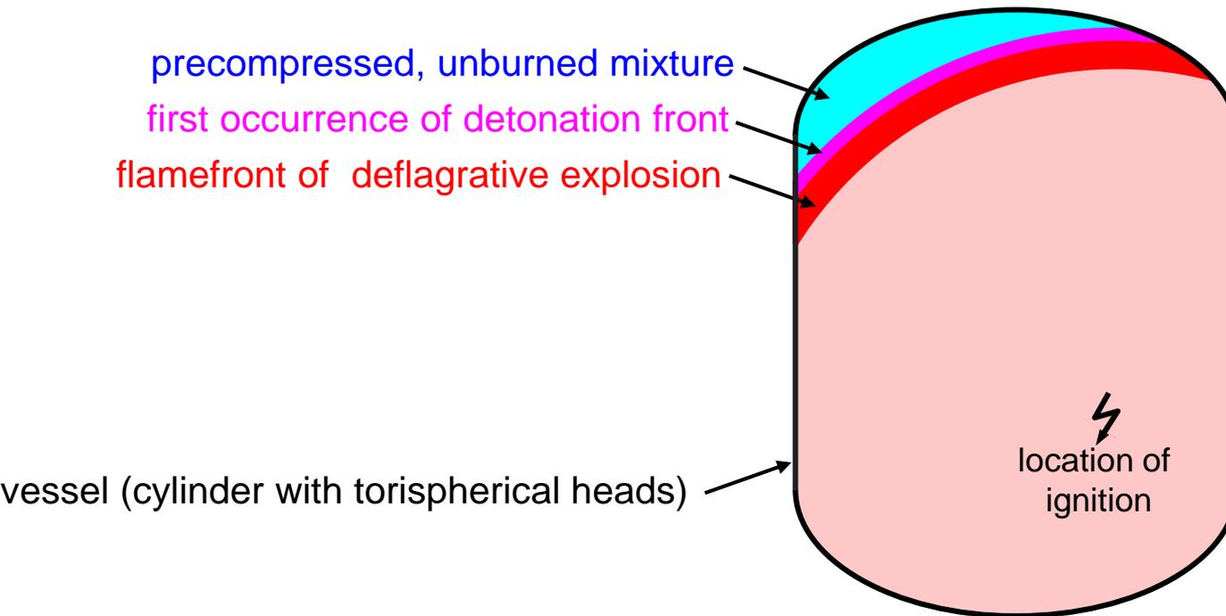
If a DDT occurs at this time instant, maximum pressure loads can be expected, because the unreacted mixture is almost precompressed to  $r \cdot p_{\text{initial}}$
