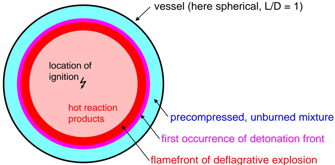
If there is a transition from deflagration to detonation in the vessel, precompression will almost always occur, because the diameter is usually not much larger than the predetonation distance. The precompression factor may attain the highest possible value, i. e. the deflagration pressure ratio.
