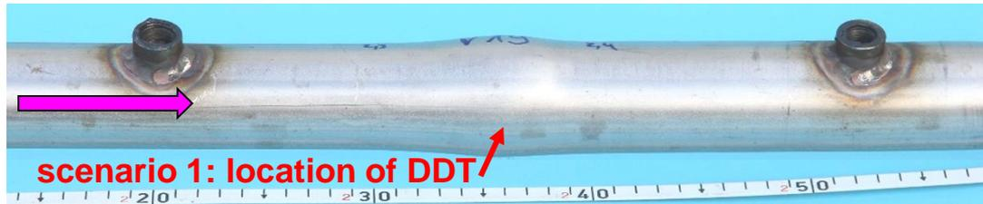
**Test 19:** 35 bar abs, 20 °C, H<sub>2</sub>:O<sub>2</sub>:N<sub>2</sub>=50:25:25 [vol.-%], 48.3x2.6-pipe, material: 1.4541
